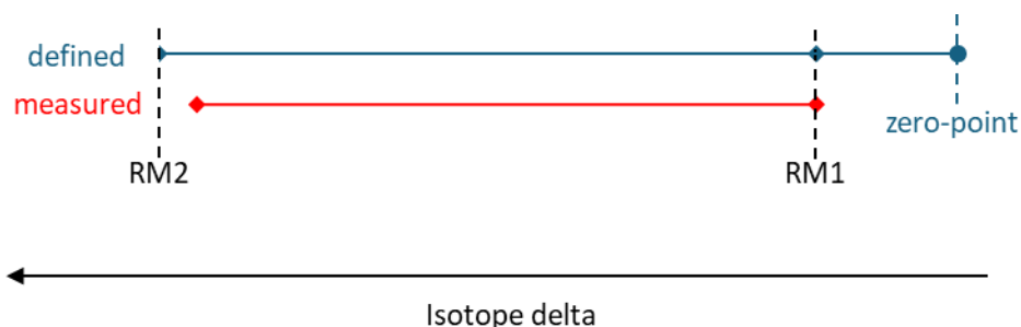
Figure 1. Illustration of scale contraction occurring during measurement of two RMs. Aligning the measured isotope delta value of RM1 to its defined value is often termed “shift” while then also ensuring the measured and defined isotope-delta values for RM2 are also aligned is often termed “stretch.” Together these processes are known as normalisation.
